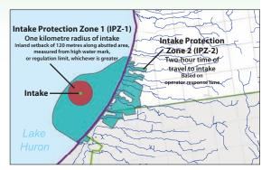
This illustration shows an intake protection zone on Lake Huron. See pages 4, 8, and 9 for ways to protect water.
